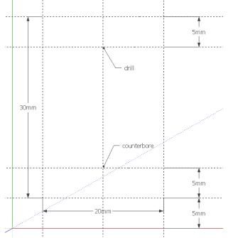
Finally I draw the part outline using the pencil and circle tools. I use the circle to cut large holes, smaller holes and countersink holes are added in SketchUCam. I finally add dimensions and comments. The final design should match your paper design.
