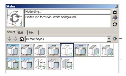
Turn the axis on as well as shading. The axis is important because the SketchUCam software will only generate g-code if the design is located entirely in the upper right quadrant. Turning shading on is also required for SketchUCam to function properly. Unless shading is on you will not be able to use SketchUCam to select objects to cut out.
